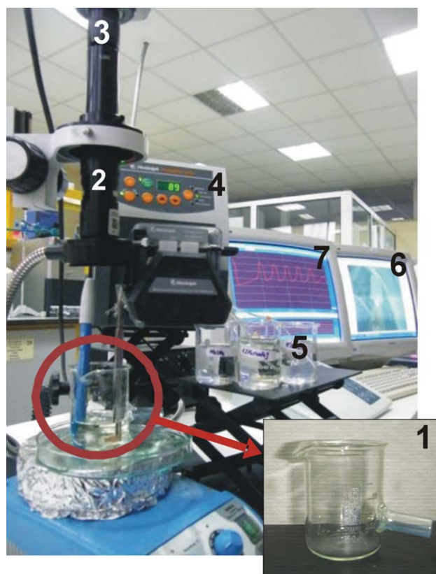
Figure 1 Experimental apparatus for real-time pH and gel size measurements during the self-oscillation of PAAc cryogels. (1): Reactor. (2): Single zoom microscope. (3): CDD digital camera. (4): Peristaltic pump. (5): Feed solutions. (6): Monitor showing real-time gel images. (7): Monitor showing real-time pH versus time data. [Color figure can be viewed in the online issue, which is available at www.interscience.wiley.com .]
